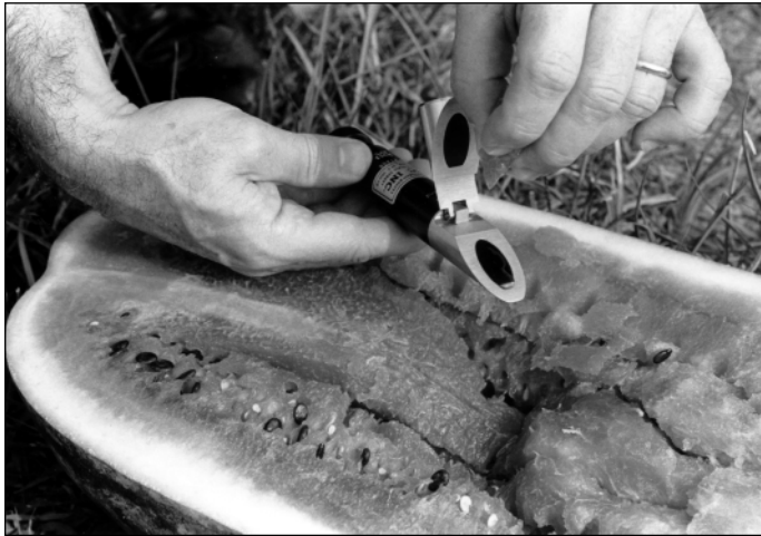
Figure 30. Use a hand refractometer to measure sweetness.
